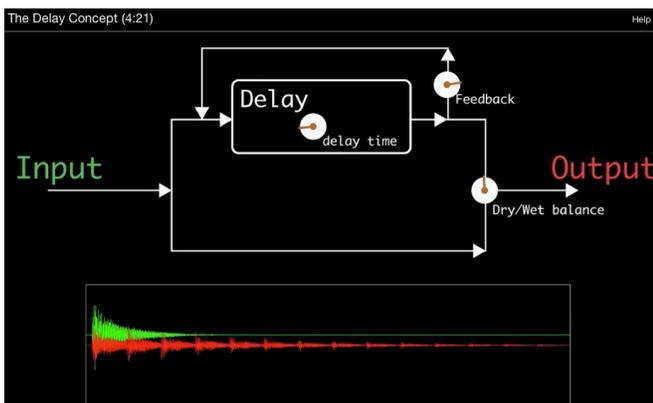
This basic functionality will translate to ALL the other delay devices that are built from this simple delay block: chorus, phasers, flangers, short and long delays, reverbs and filter devices.
