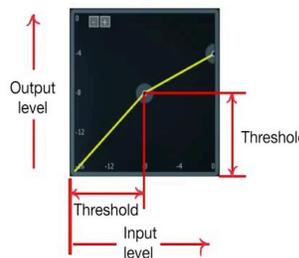
A transfer function diagram shows how input level relates to output level.
