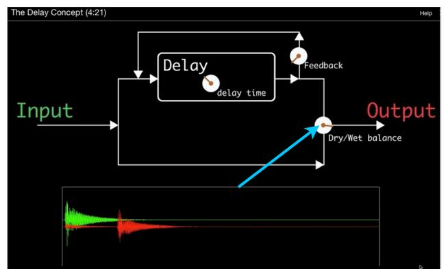
The **FEEDBACK** control routes some of the output of the delay block back to the input of the delay block. It is only a **Gain Stage**. It's increasing the level of the signal going back to the input of
