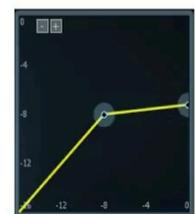
At 10 : 1 a compressor output is one tenth the input above the threshold. The compression is so extreme we call this a limiter.
