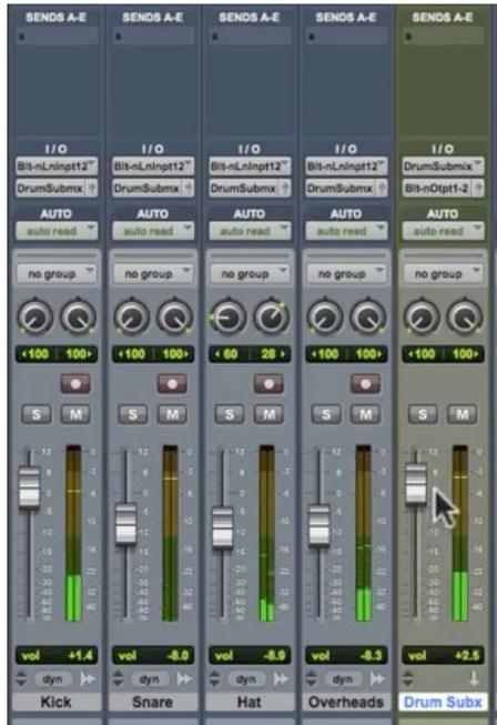
that **Drum Submix** Bus. Use a single insert like an EQ or compressor, effecting all the drums as a single unit. A single fader now represents the entire Drum Kit.
