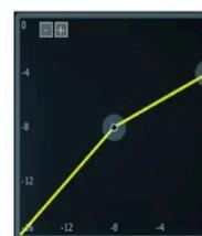
At 2 : 1 a compressor output is half the input above the threshold.
